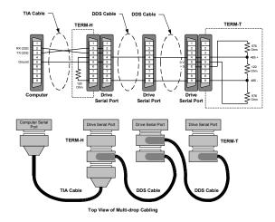
Figure 32: Multi-Drop Wiring Pinout
